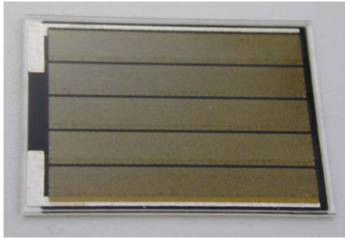
Figure C.1: Panasonic (BP-243318) solar cell chosen for the solar power train.
