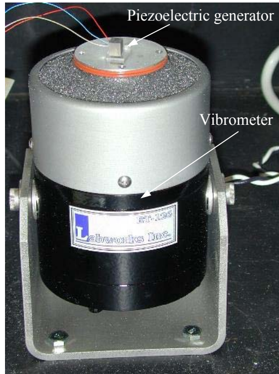
Figure 5.3: Vibrometer with test generator mounted.
