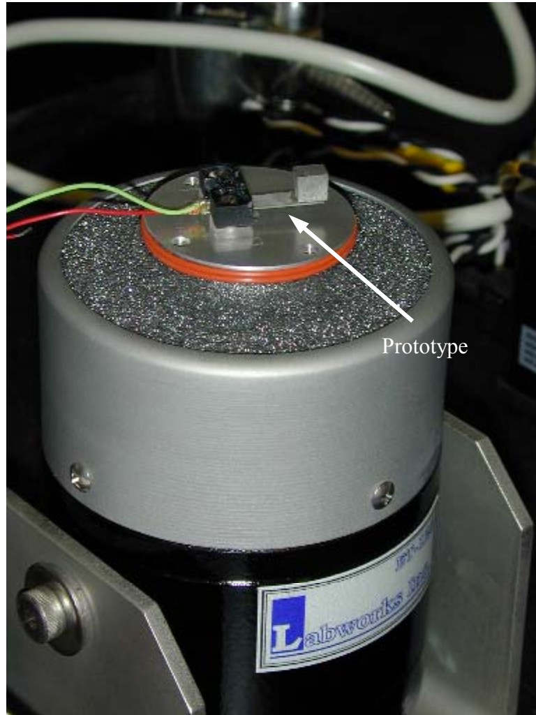
Figure 10: First piezoelectric prototype mounted to the vibrometer for testing
