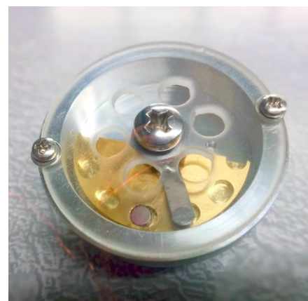
Figure 5. Photo of the piezoelectric rotational harvester prototype (with one beam)
